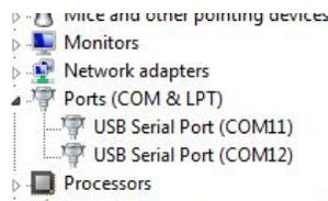
The Telescope Interface Module provides two virtual COM ports; one COM Port is used for remote operation whereas the second COM port is used for fail-safe firmware update. The user should try to establish communication using the lower COM port first; if this is not successful, please use the other COM port.
