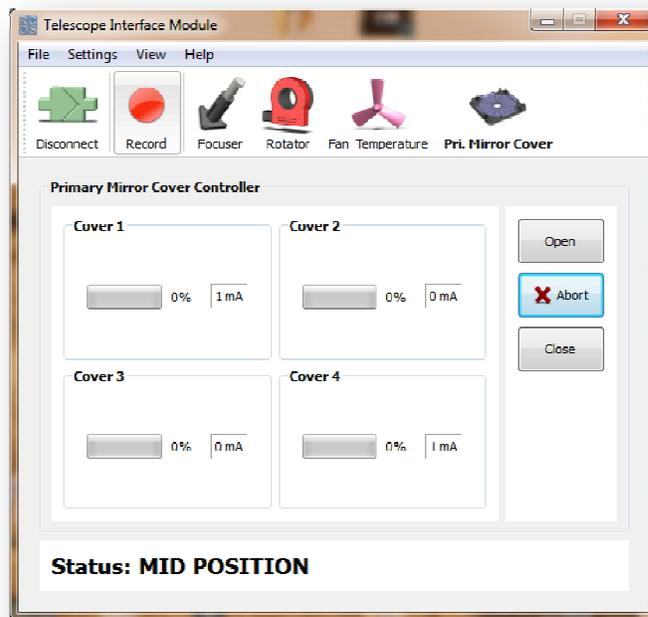
The cover-flap controller allows the user to remotely open or close the mirror cover if they have been installed. Otherwise, this dialog pane can be disabled in the menu [view->show Pri. Mirror Cover Tab]. The user can specify the flap speed in the settings dialog - please refer to the settings section in this manual.
