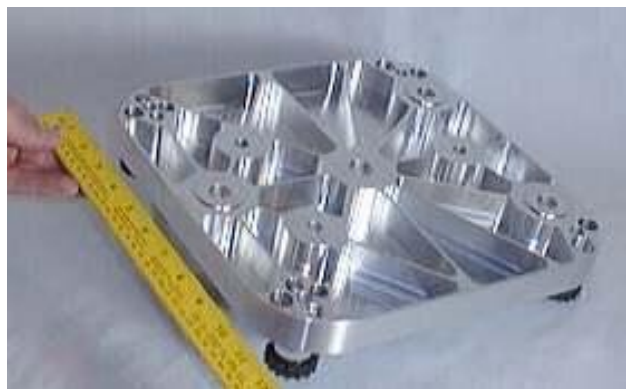
Figure 62: Bottom view of the unanodized lightweight Base Plate
