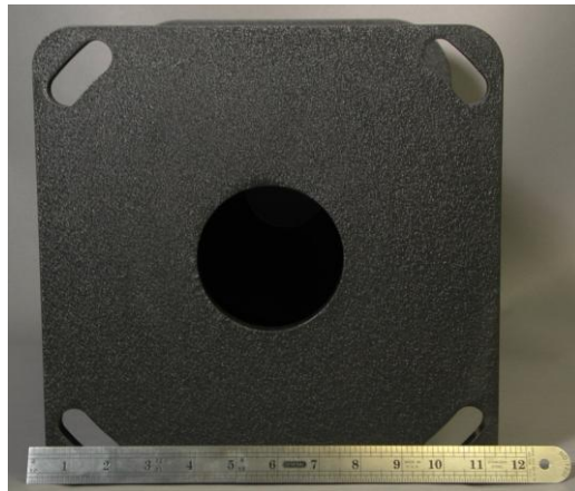
Figure 68: Photograph of pier base plate. Note slotted holes.
