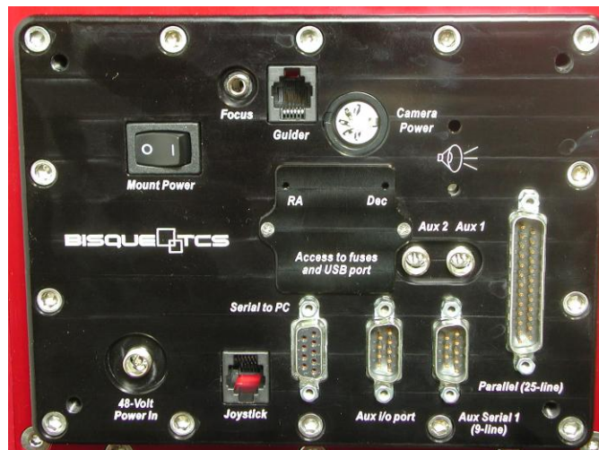
Figure 83: Use a small Phillips screwdriver to remove the cover labeled “Access to Fuses and USB Port” to access the USB port.
