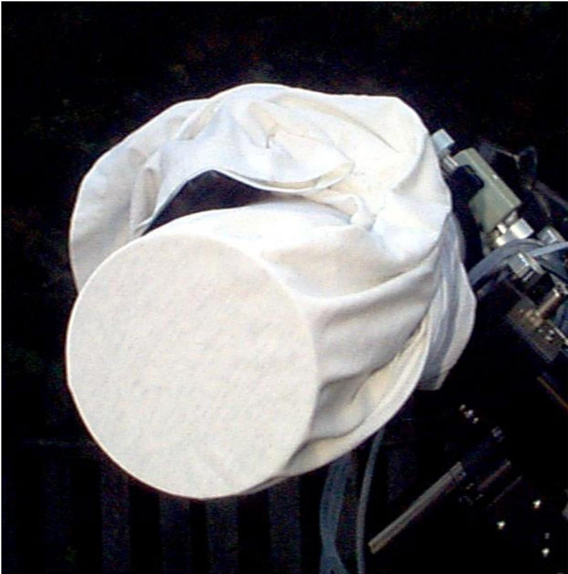
**Figure 234: Using a T-shirt to take a flat in daylight. Be sure to point the scope away from bright sources of light.**
