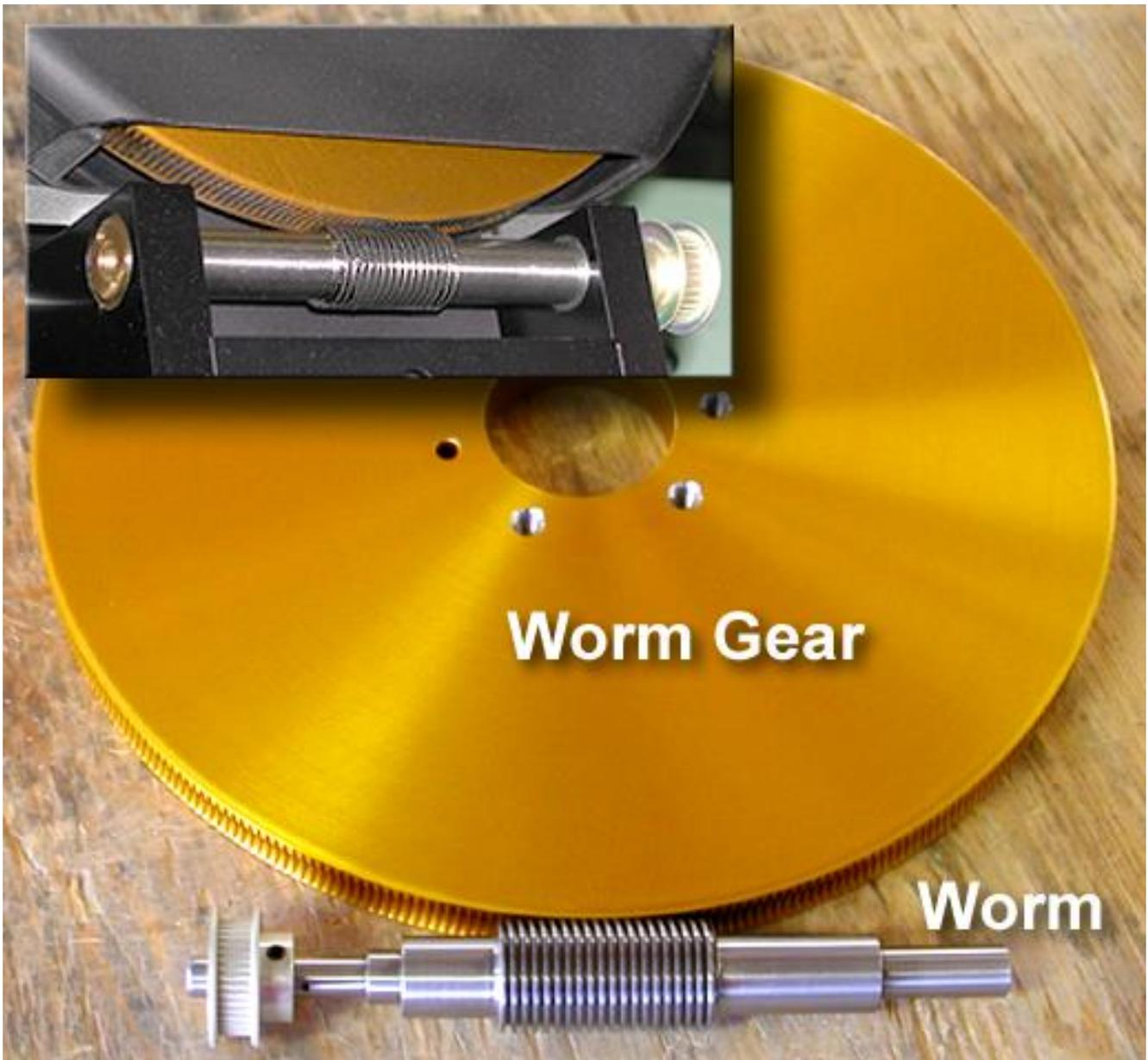
**Figure 213: A Byers precision worm and worm gear.**
