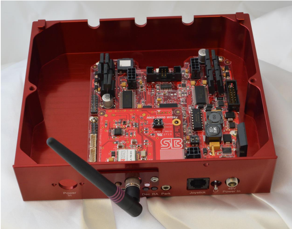
Figure 15: WiSky board installed on the MKS 5000 PCB with the antenna and WiSky expansion bus cover installed.
