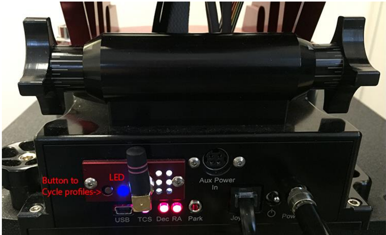
Figure 33: The WiSky's Profile LED glows with a steady dark blue when configured for the default ad hoc network profile.
